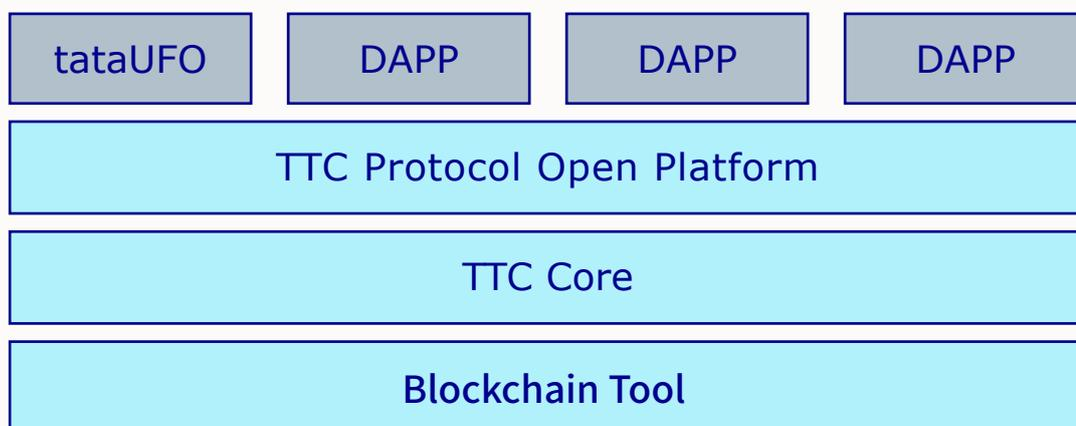
Figure 9. The technical architecture of the TTC Protocol
